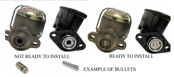
IMPORTANT! MAKE SURE YOUR MASTER CYLINDER IS READY TO BE INSTALLED ON HYDRO UNIT! DO NOT USE ANY DEEP BORE MASTER. SEE EXAMPLES ABOVE. WH MULTI APPLICATION MASTERS HAVE A "BULLET" TO INSTALL IN THE BORE OF THE MASTER. MAKE SURE THE "BULLET" IS INSTALLED TO KEEP FROM DAMAGING THE NEW UNIT!
