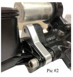
Install the brake pedal push rod and adjust the brake pedal height by spinning the brake pedal push rod. The push rod assembly must thread on a minimum of 3/4". Once you have the desired brake pedal height install the brake pedal rod, brake light switch and bushing to the brake pedal with retaining clip/pin. Double check for appropriate thread engagement at brake pedal push rod, then tighten the brake pedal push rod jam nut firmly. Reconnect the brake light switch electrical connector.
